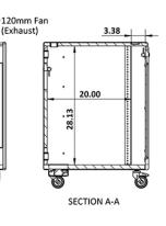
The mobile rack model **REX16** includes front and rear 16U rack rails for equipment up to 20" deep, framed front door with a tinted acrylic window and heavy duty casters for easy maneuverability.
